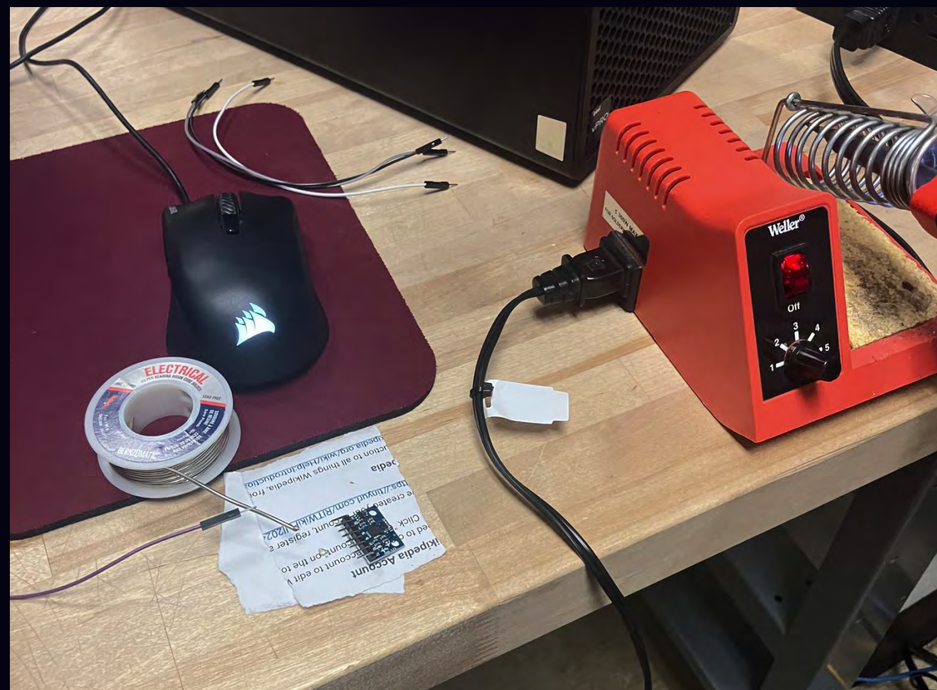
Soldering the IMU pins.
